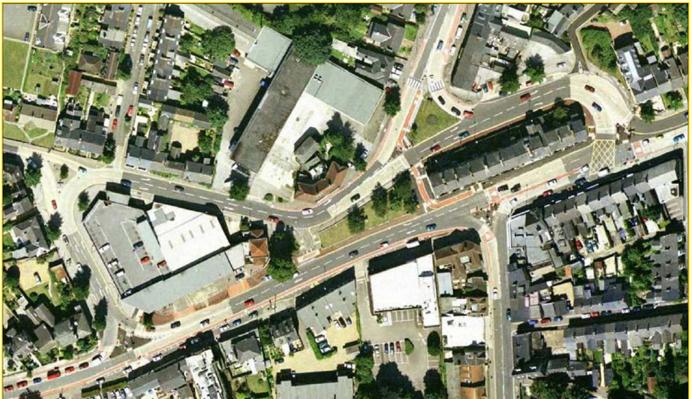
Aerial photo, showing anti skid surfacing (tan) and cycle facilities (pink) as part of the Mitchams Corner scheme
