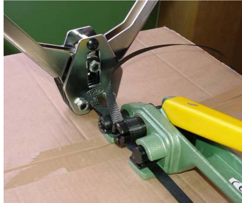
Crimp the seal into place.
