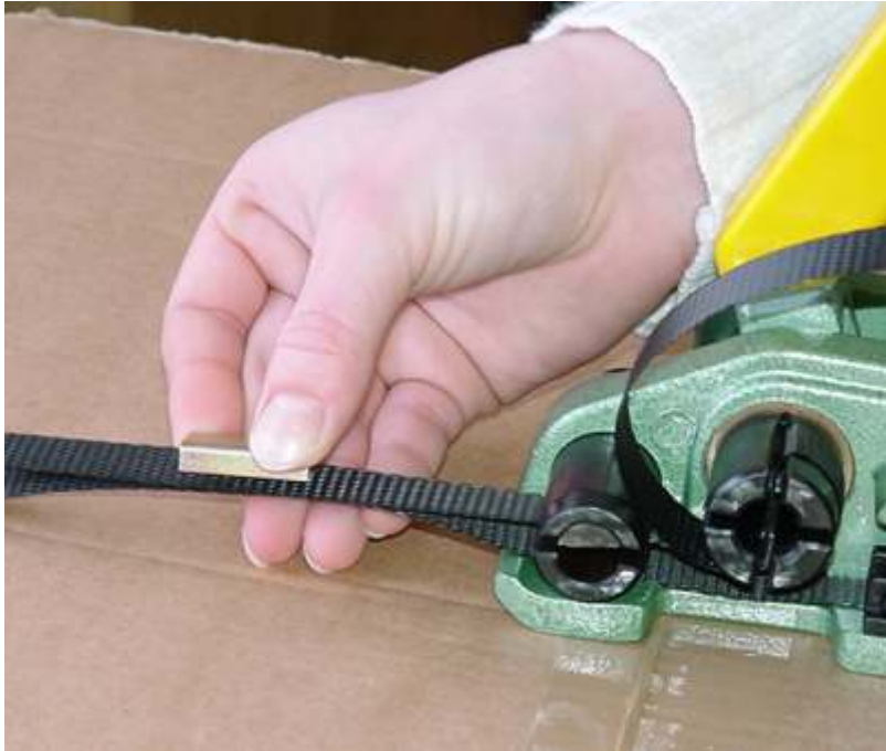
Clip the seal over the strap where they run one above the other.
