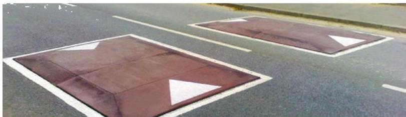
A speed cushion is a short, raised, rounded device, normally in the centre of a road lane. Speed cushions are designed to be slightly wider than a car, so car drivers need to slow down and drive over the centre of the speed cushion to reduce discomfort. Buses are wider than cars, so they can drive over speed cushions without passengers feeling anything. In Cambridgeshire, speed cushions are normally 1.6m-1.8m wide.
